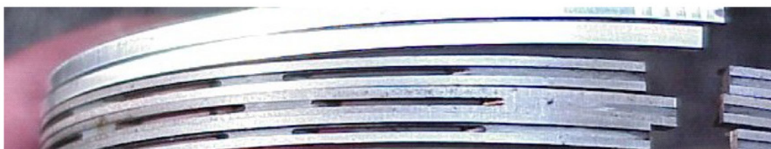
THE RAILS OF THE OIL RINGS HAVE BEEN WORN AWAY, COMPARE THE APPEARANCE WITH A NEW OIL RING SHOWN BELOW
