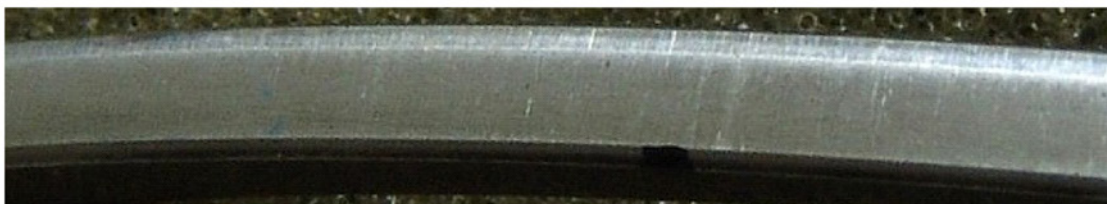
THE FACES OF THESE COMPRESSION RINGS EXHIBIT FINE VERTICAL SCRATCHES
