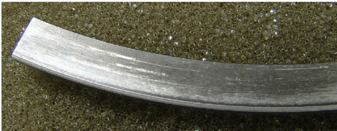
THE SIDE OF THIS COMPRESSION RING HAS BEEN DAMAGED BY CONTAMINATION AS THE RING ROTATED IN THE RING GROOVE IN THE PISTON
