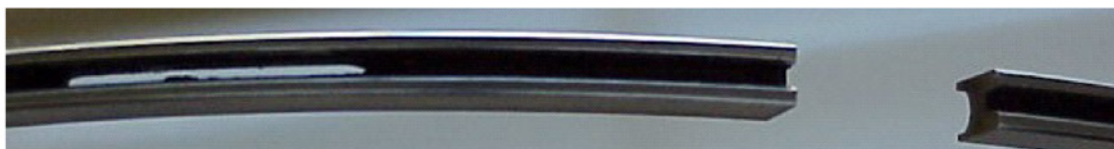
THE RAILS OF THE OIL RINGS HAVE BEEN WORN AWAY, COMPARE THE APPEARANCE WITH A NEW OIL RING SHOWN BELOW
