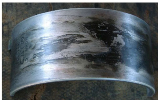
Oil has worked its way into the space between the two surfaces and resulted in these markings.
