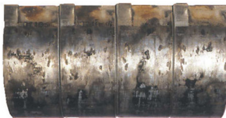
Fretting and polishing due to movement.
