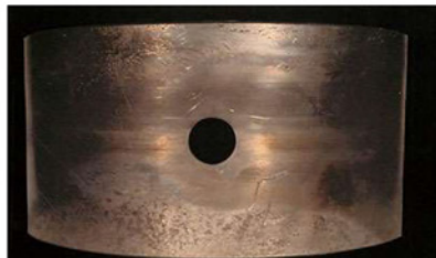
Wear pattern created on the back of the bearing due to the movement.
