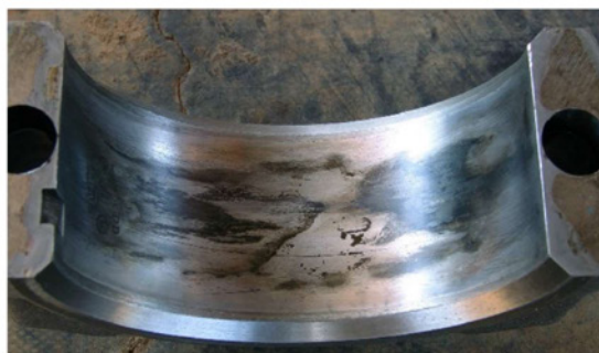
Oil has worked its way into the space between the two surfaces and resulted in these markings.
