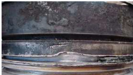
Initial damage from a broken ring
