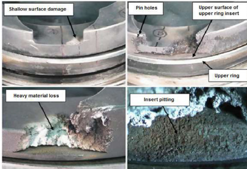
Piston OD visual damage. Note the heavy material loss working in from the OD, but no ring damage.
