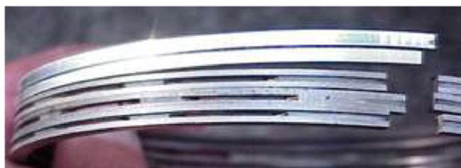
The appearance of three oil rings which have been considerably worn by abrasive contamination.
