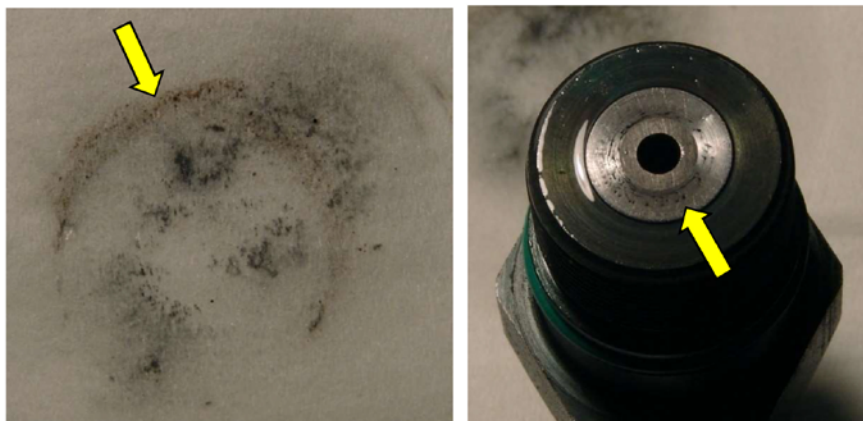
Contamination found inside the injector
