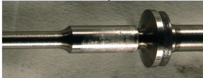
The resultant damage to the needle
