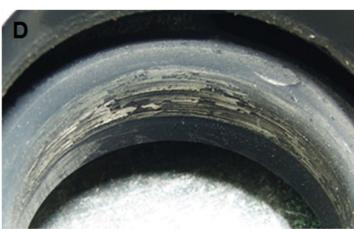
**Ingestion of foreign object** can account for as much as 40% of turbocharger failures and the culprit can have a number of origins, a piece of burnt or broken valve exiting the engine through the exhaust will end up damaging the turbine wheel, damaged pistons or piston rings could also be a source.
